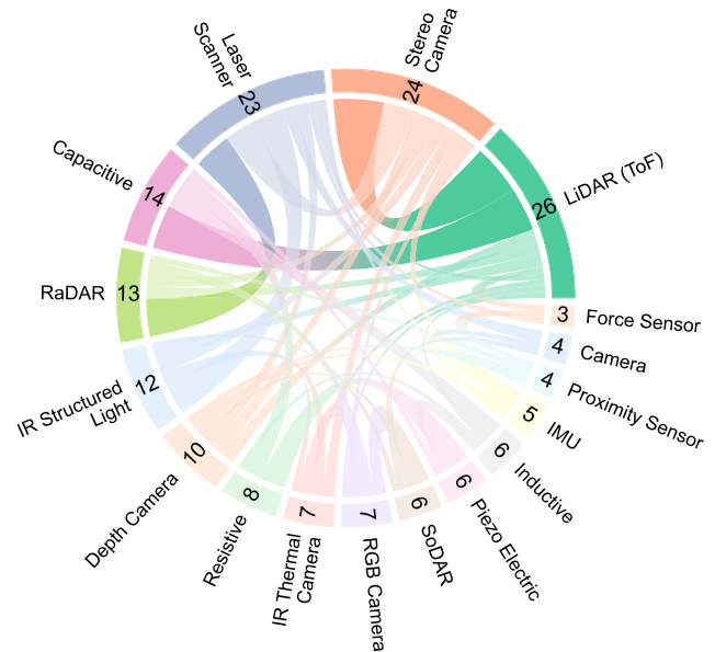
Fig. 15. Chord diagram visualizing interconnections among the most used sensors (with more than five combinations) within a safety system, with the line thickness representing the relative frequency of each sensor pairing. Notably, the connections between LiDAR (ToF) and stereo cameras, LiDAR (ToF) and capacitive sensors, as well as laser scanners and RaDAR, are most prominent, illustrating key sensor synergies.
