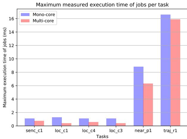
Fig. 1. Maximum measured execution times of the main recurring tasks of the Thales application on the SABRE Lite.
